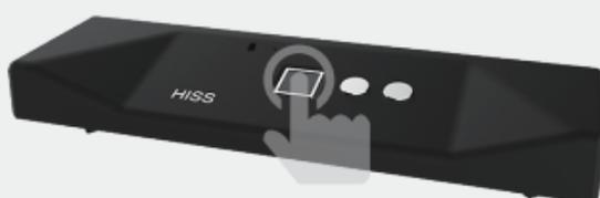
Please put your finger on the fingerprint, when hear the beeping sound, and the light turns green. Remove your finger and put the same finger on the fingerprint again. After hearing the three beeping sound, remove your finger.
